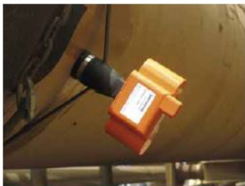
Figure 5. Installing Permasense ultrasonic corrosion sensors is a simple matter. Approximately 25 sensors can be installed in one day per installation technician.
